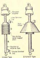
Fig. 166.—The "cupped-discgap" protector. (Westinghouse Elec. Mfg. Company.)
